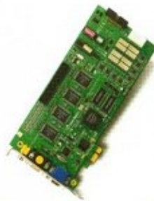
PCI Express Dsub - Type 212 (W) x 99 (H) mm
