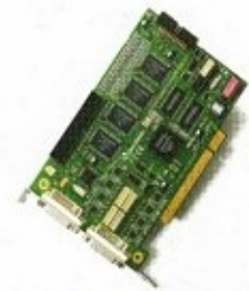
PCI DVI - Type 165 (W) x 95 (H) mm
